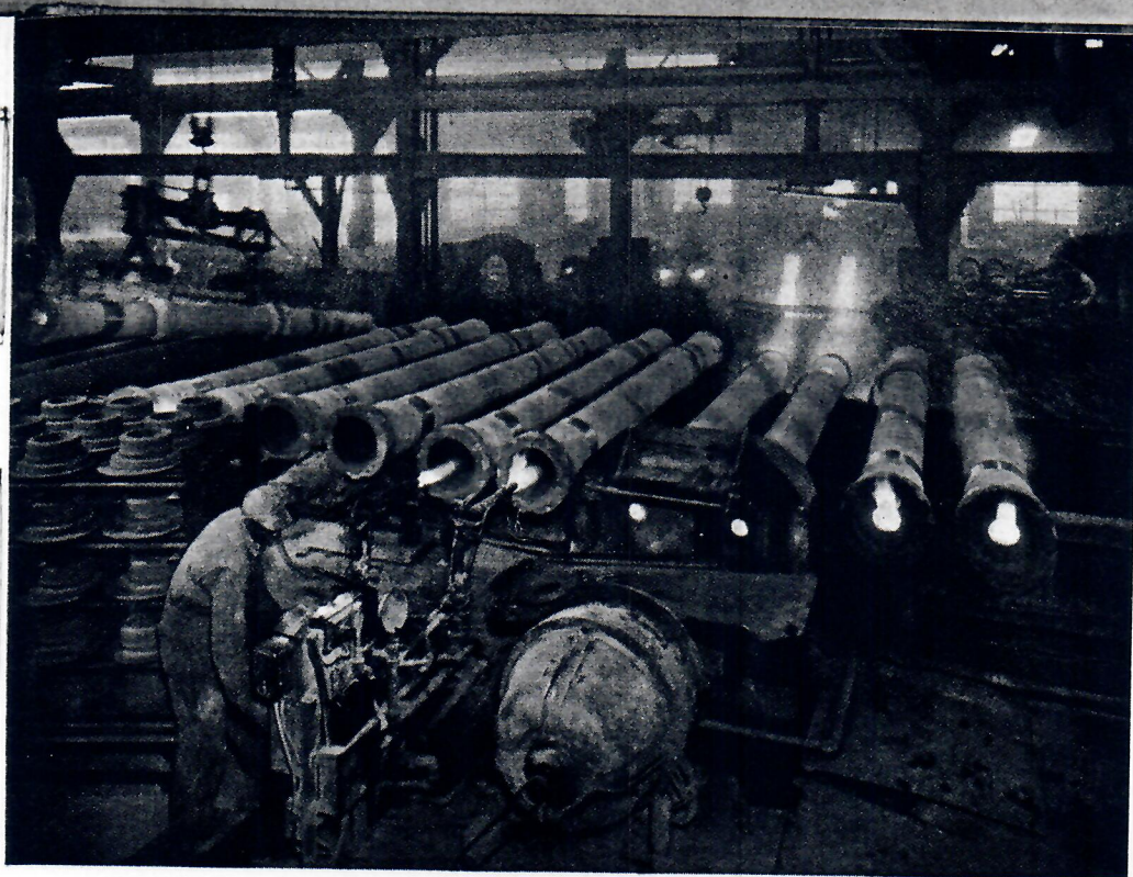
The casting of SAND-SPUN pipe by the centrifugal process.
